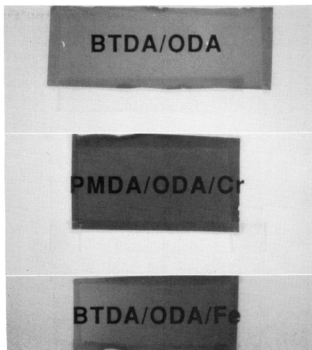
Figure 2. Photographs of free-standing polymer films of BTDA-ODA, PMDA-ODA/Cr, and BTDA-ODA/Fe.
